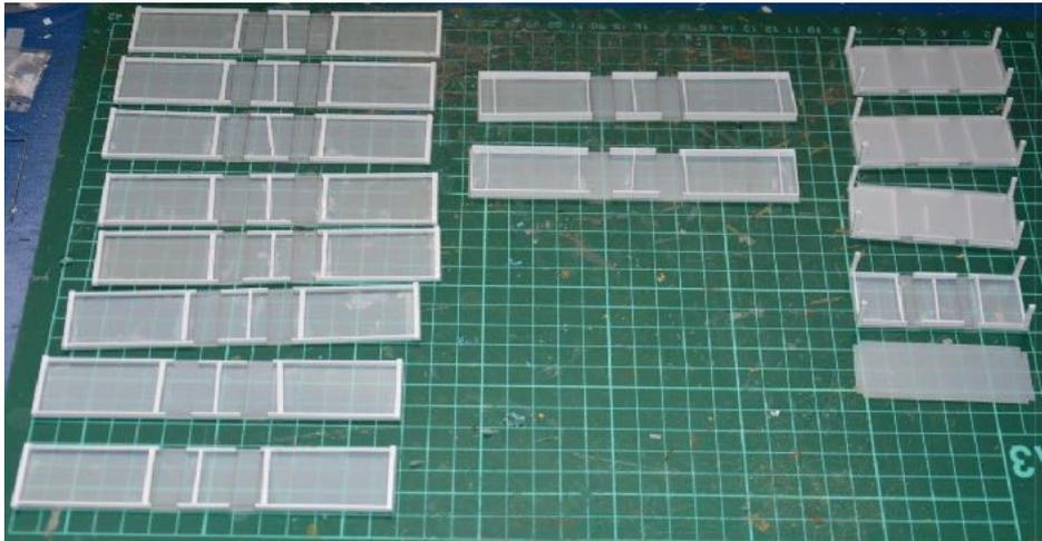
The half- height containers were built using Evergreen # 154 - •060": x •080" styrene for corner post and the base sides I use the •080" side of the strip, •030" sheet styrene was used for the ends and
