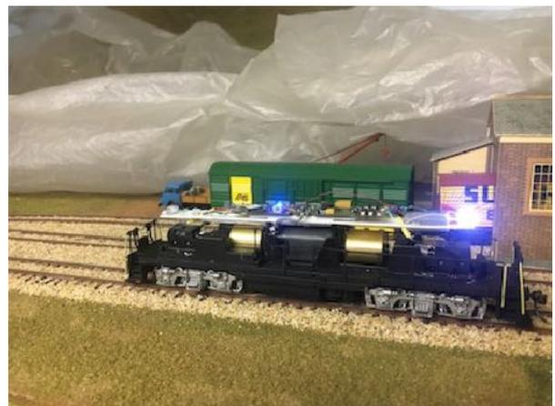
*Above: 436 is almost finished. The shell has had the first of two coats of Vallejo acrylic clear matt. The Soundtraxx Economi decoder has been installed along with a sugar cube speaker from OzRail. I removed the original printed circuit board that was fixed to the top of the motor cradles and replaced it with 1.5mm styrene with a stiffener and mounted the decoder speaker and LEDs on the styrene. I have test run the install in 436. Click video link below to see.*
