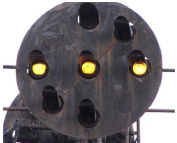
A prototype PRR position light signal head showing three horizontal lights, which indicates STOP.
