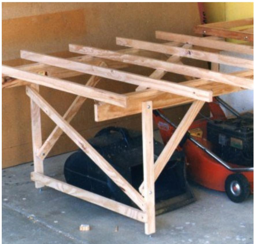
The fully braced leg system built out of 42 mm by 19 mm pine shown in the attached photo can support layouts with decking up to 1,200 mm high.
