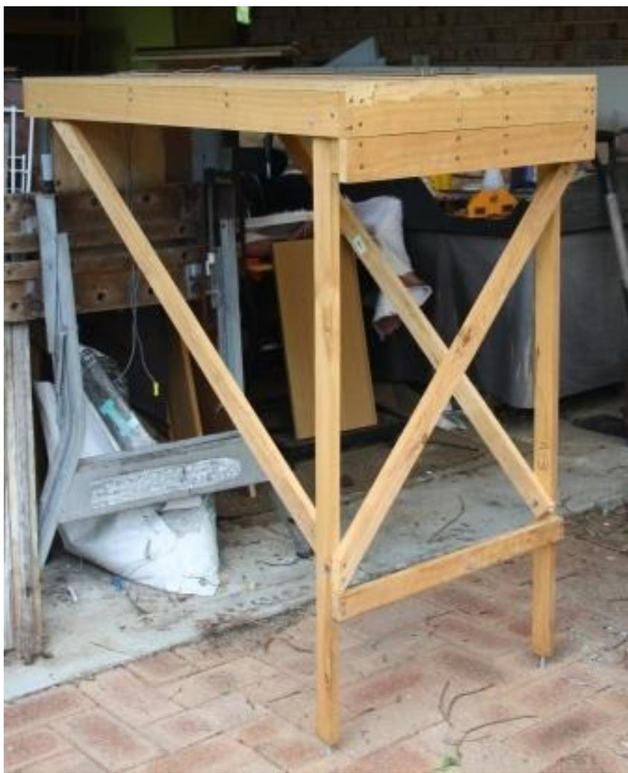
Floors are seldom level. Drilling the bottom end of your layout legs and fitting a 6 mm hexagon head coach screw to each leg or Tee nuts, allows you to level your layout as you install it. If your layout room is carpeted a 100 mm square of plywood as shown in the photo will prevent the coach screw damaging the carpet and allow for later height adjustment.
