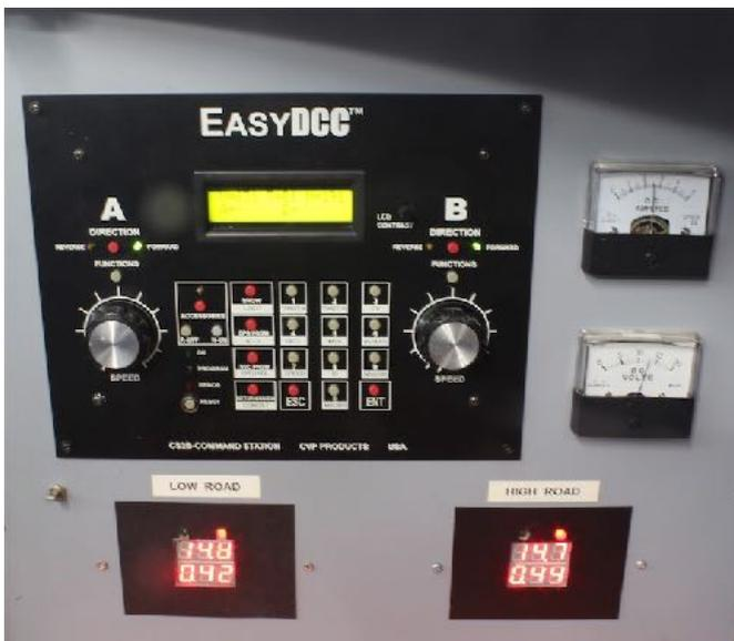
voltage of 14.6 volts. This is verified by two Rampmeters that give constant readings of the power buss. A computer is connected to the command station and runs a program JMRI which has many sub systems for model railroaders. I use one - Decoder Pro, this is for testing and programming the decoders in each of the locos. The computer is also connected to a programme track through a Sprog 3 unit.
