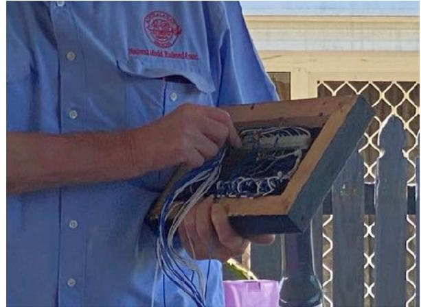
Jack drafted the track diagram using Excel and then had his local engraver engrave the control panel accordingly. The black on white is amazing. This allows pre wiring of the control panel at the tool bench and makes for easier under the layout installation.
