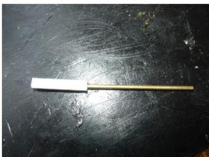
Glue the brass tube into the styrene tube flush with the bottom.
