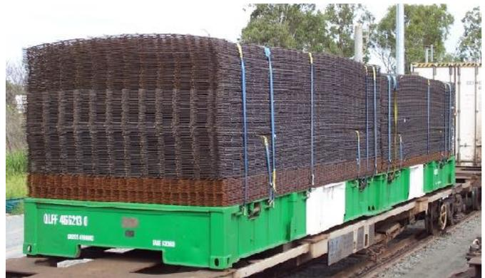
**2** No end gates and secured by 2t Web Strap
