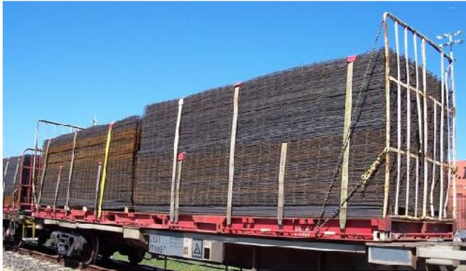
**1** Has end gates & secured by 5t Web Straps
