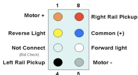
To the left;- this shows the pin arrangement and their assignment and colour.
