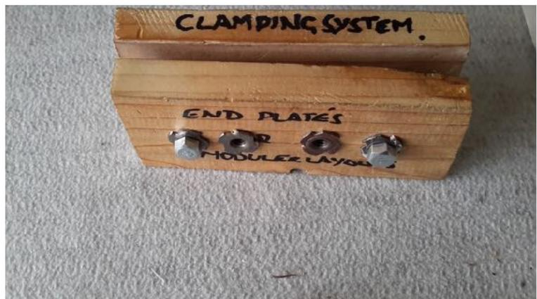
**2** Example of Bolt and Tang placement on End Plates
