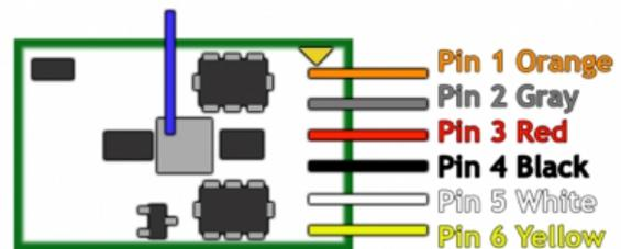
This sort of connection comes in handy for models in other scales. The Blue wire can be left unconnected and the + side of the function is connected to a track pickup - this is why I always put the resistor for LEDs in the function control wire. This requires running one less wire between loco and tender when installing in a brass type loco.....
