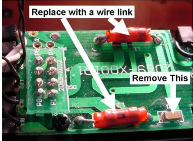
**1** Remove the 8 pin plug (on the left). Remove the two red components resistors) and replace with a wire link. Remove the small capacitor as indicated.
