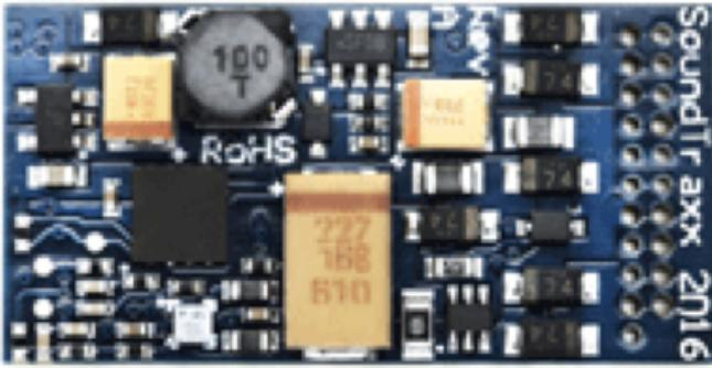
TSUNAMI 2 Has 6 output Functions
