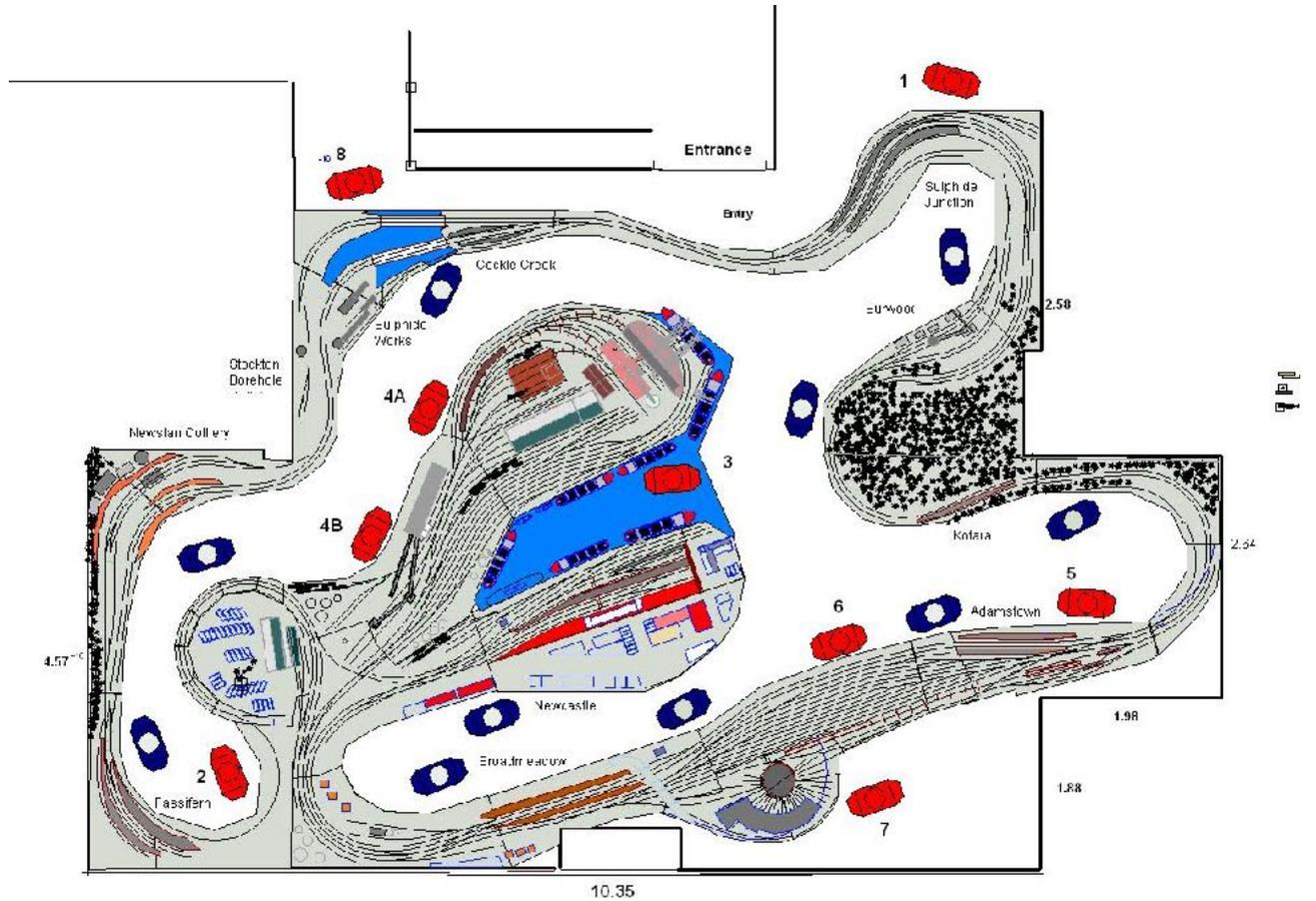
**4** Layout Plan as at 2016. Some changes have been made since. Overall Dimensions 12.33m by 8.15m
