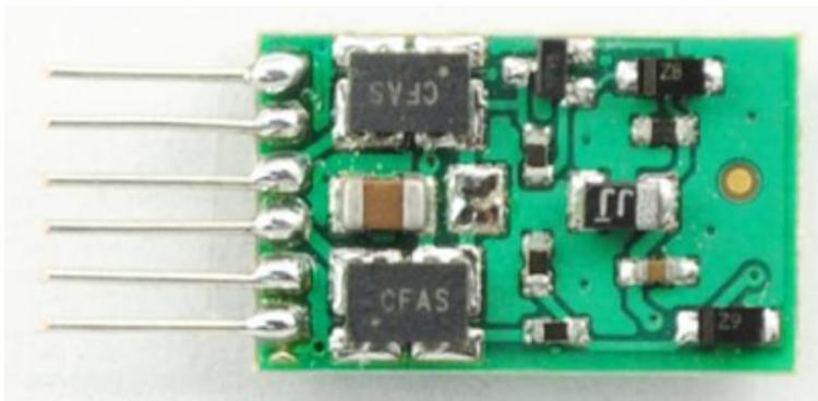
Not to be outdone, N scalers have the 6 pin decoder. A six pin decoder brings the Question - does it have the usual 2 light outputs white and yellow. The answer is "YES" and it is pointed out that there are only 6 wires. 2 = track pickup, 2 = motor connection and 1 for the headlight and 1 for backup light. In this case the "positive" side of the function is connected to one of the track pins.
