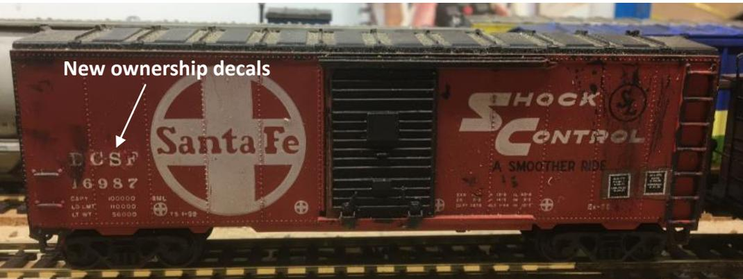
The reporting marks on freight cars and cabooses are easily scraped off with an angled hobby knife blade. Decal reporting marks of the same type face as the model originally carried give the model a new identity.
