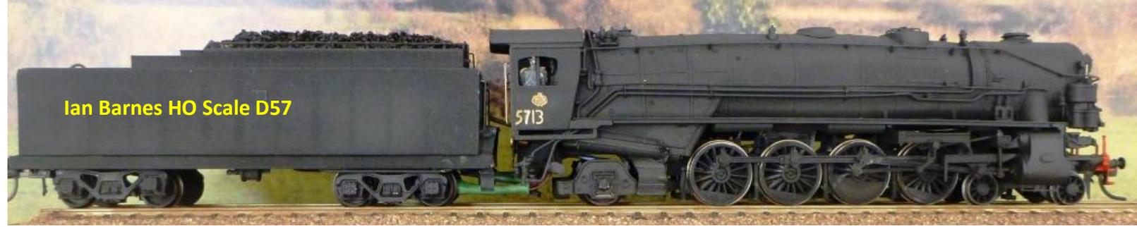
otive. It was 99.5% assembled with solder. He only used CCA to attach the smoke box. This allows him to replace the LED headlight if required. He has installed a sound decoder in the tender beneath a removable coal load. Whilst the whistle isn't quite right "German style" it will suffice for the present.
