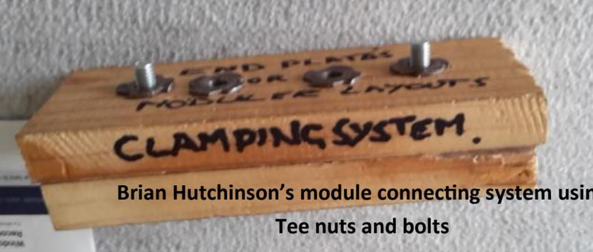
**Brian Hutchinson's module connecting system using Tee nuts and bolts**
