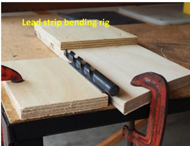
Step 5: I devised a basic jig to put a mild curve in the lead sheet. This was by using 2 small pieces of plywood clamped to the work bench parallel to each other with a gap slightly smaller than the width of the lead strip.
