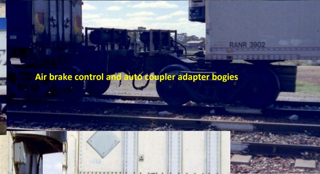
Air brake control and auto coupler adapter bogies
