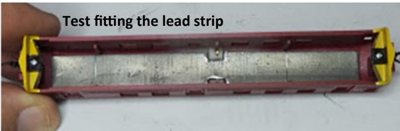
Step 7: Next I added as much lead weight as possible to the chassis. Here the lead strip is cut to fit inside the shell and then hot glued to the top of the gearbox. I added as much weight as the space would allow
