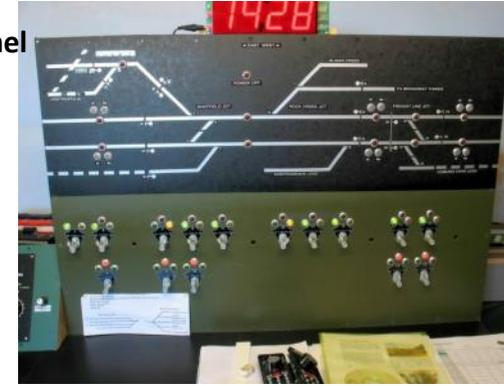
full logic in the program to provide all of the features of the CTC systems used in the 1970's. He did not want a 'modern' control system, but rather the familiar old 1940's style Union Switch & Signal CTC panel. For example, a signal cannot be cleared unless the switches are set correctly, and there is no opposing movement and there is no train in the block.
