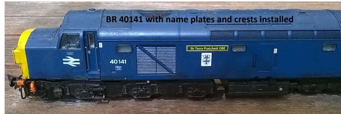
The name plates and coats of arms were printed using an ink jet printer on 80 grams per square metre paper (photo copier paper). Once the ink was dry the printed name plates and coats of arms were sealed both sides with acrylic matte medium and allowed to cure. The name plates and coats of arms were secured to the model with acrylic matte medium
