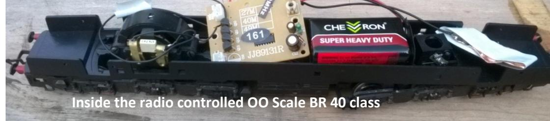
I tried two AA dry cell batteries but they wouldn't budge the Lima motor. In desperation I tried a nine volt battery. This worked well. (No smoke!) With a little wriggling I installed the receiver circuit board from the pickup, the nine volt battery and the attendant wiring into the 40 class and reinstalled the body shell. On the layout the model sailed along at a sedate speed. This was a considerable improvement on my previous attempts to operate this model on DC track power. I was in business.
