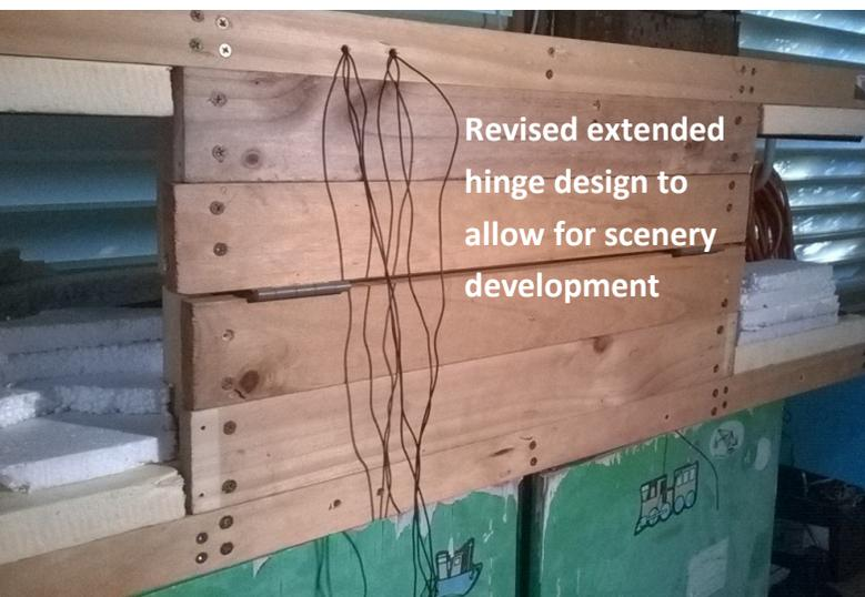
secured to the layout framing by lengths of 68 mm by 19 mm pine
