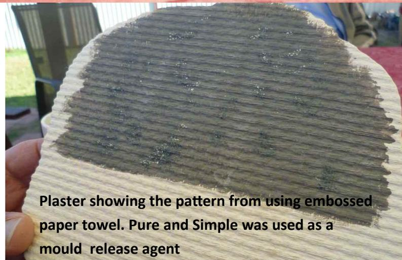
Plaster showing the pattern from using embossed paper towel. Pure and Simple was used as a mould release agent
