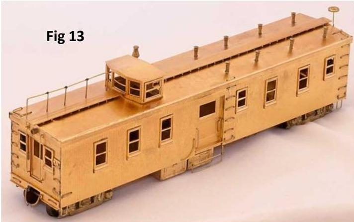
Fig 13 is the roof of the model as acquired, eight vents where there should only be five, no cupola handrail and no roof walk around the cupola. The handrail as already stated was completely wrong.
