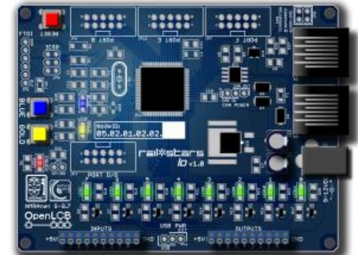
The bus cable specified by the LCC standard is the readily available, or fabricate it yourself, computer or LAN (Cat 5) cable with standard RJ45 connectors on each end.
