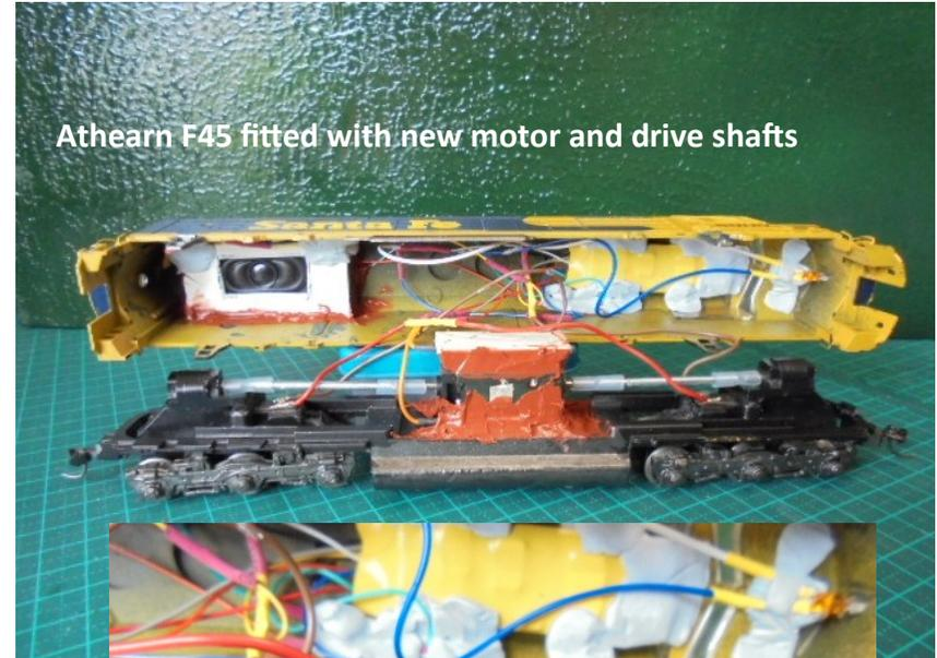
Athearn F45 fitted with new motor and drive shafts
