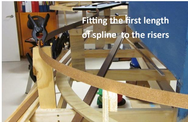
in PVA white glue. This glue was spread with an old paint brush. Then this length was attached to the first spline and clamped
