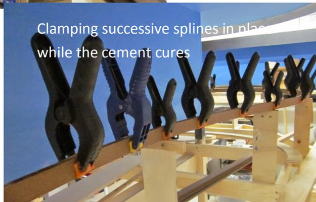
Clamping successive splines in place while the cement cures
