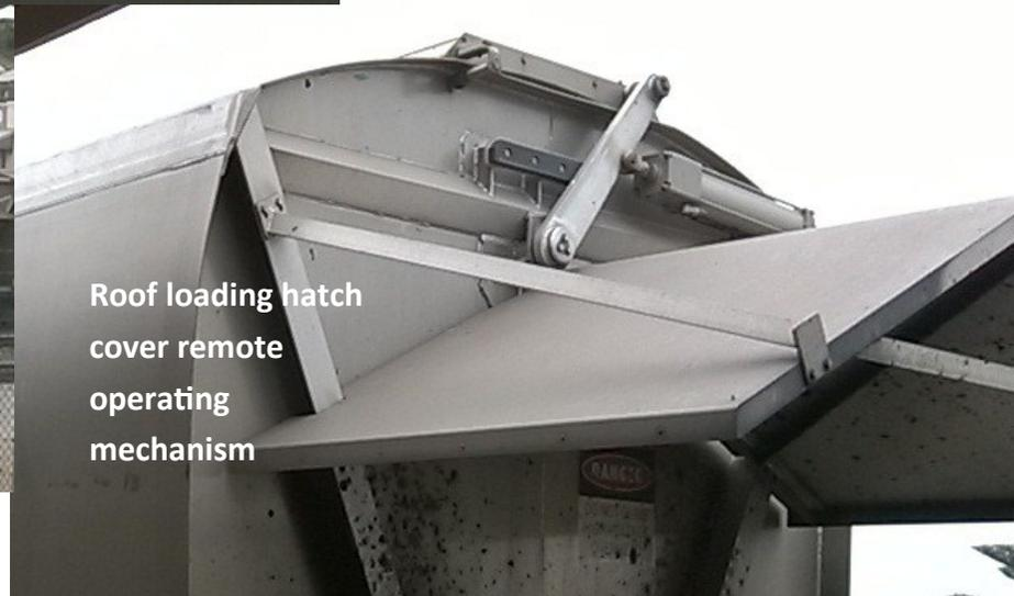
Roof loading hatch cover remote operating mechanism
