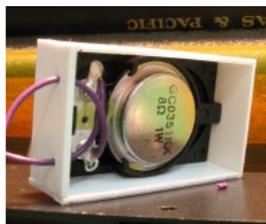
Speaker box made from 1mm styrene, the back cover will be added. No technobabble – your speaker needs a box! The volume should be set so that you can hear the loco from no more than six feet away (500ft, 160m). So adjust CV1xx to 150 for starters, then up or down by 10 until you have the right volume.
