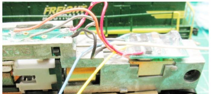
In all cases I use 820 ohm resistors for this type of application. Remember the longer lead on the LED goes to the Blue wire from the decoder.
