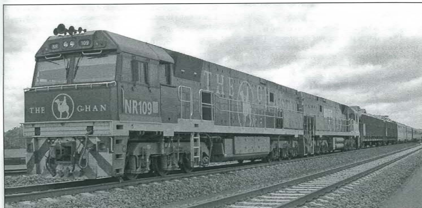
The Ghan at Katherine pulled by NR 109 and NR 29. Both locomotives are Goninan/General Electric CV40-9i locomotives weighing 132 tonnes and developing 3000 kw.
