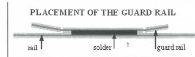
To complete the turnout, cut two lengths of rail for the guard rails. Scrap lengths are great for these. With the pliers slightly bend each end of these guard rails. Clean the inside edge of the rail, apply flux and a good run of solder. Do the same on the inside of the rails where the guard rails will be located. Place a
