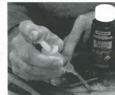
Apply flux with a needle
