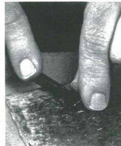
Cutting resin-core solder
