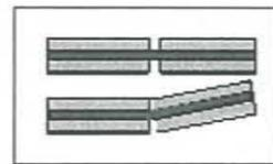
and allows the rail to bend sharply. Before doing anything else to this rail, repeat the process with the curved rail. On both these rails, clean, flux and add solder to the inside of the guard rail section of the wing rails. See the diagram opposite. These areas of solder should match the solder applied to the outside of the frog rails (see Step 4 - The Frog) Now to fit the straight wing rail. Lay the steel ruler against
