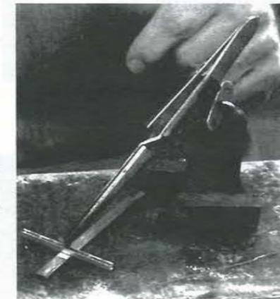
end pressure of the tweezers [locked into the 3<sup>rd</sup> hand] on top of the pieces to be soldered. Because in this technique you do not need to touch the pieces to be soldered you will only need enough pressure to stabilise the work piece, which requires very little pressure]
